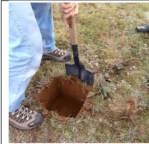
Figura 38a. Excavating a square hole (20x20x20cm deep) to assess the macrofauna in this volume.
