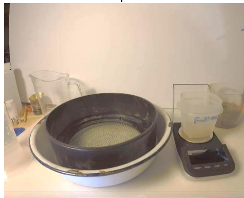
Figure 17. Preparing to wet-sieve the particulate organic matter (POM) out of soil, with the 2 mm sieve submerged in the pan of water.
