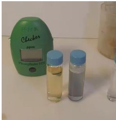
Figure 36. A blue color will develop in the extract with the reagent packet added. The other yellow colored vial serves as the color blank to be measured in the colorimeter.
