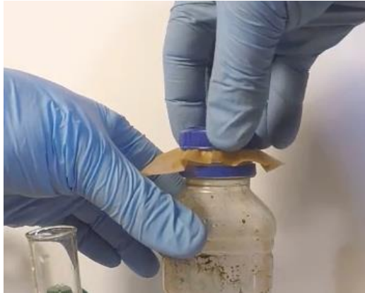
Figure 30. Placing a double layer of coffee filter paper below the lid of the bottle.
