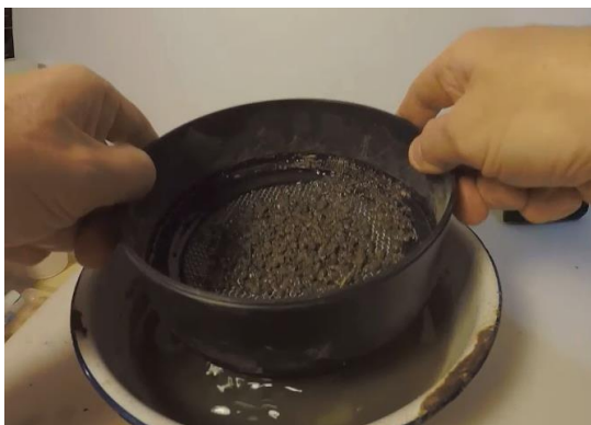
Figure 13. Lowering and raising the sieve 50 times in two minutes.
