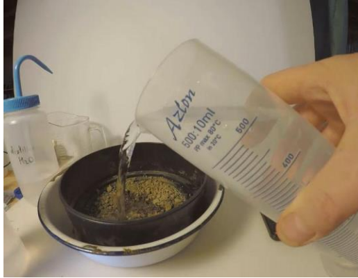
Figure 19. Adding water to the sieve and soil before wet-sieving (note: the graduated cylinder is just a convenient container, it is not necessary to precisely measure the water)
