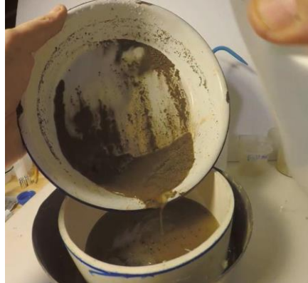
Figure 20. Transferring the material which passed the 2 mm sieve to the 250 micron sieve.
