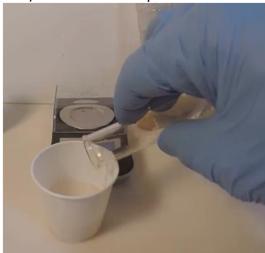
Figure 33. Mixing 3 mL solution of sodium bisulfate (15g NaHSO 4 per 100 mL) to acidify 7 mL of filtered extract. Note the bubbling of the soil extract as bicarbonate reacts with the acidic bisulfate.
