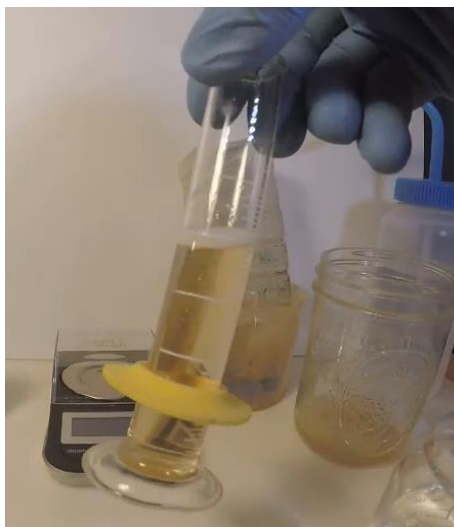
Figure 34. The extracted, filtered solution has been acidified and brought to a standard volume of 20 mL. It is ready for reacting with the color reagent to develop the blue color and then read with the colorimeter.
