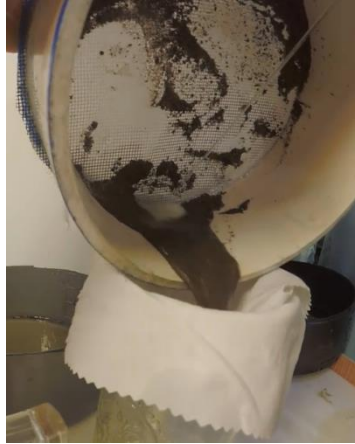
Figure 15. Washing a stable aggregate fraction from the sieve to a funnel with a cloth to retain the soil for drying and weighing.
