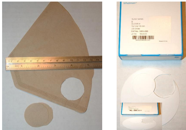
Fig. 4. Left: cone coffee filters; Right: lab-quality filters, Whatman type #5 with 2.5 micron pores. Circles with diameter ~3cm can be cut for filtering soils.
