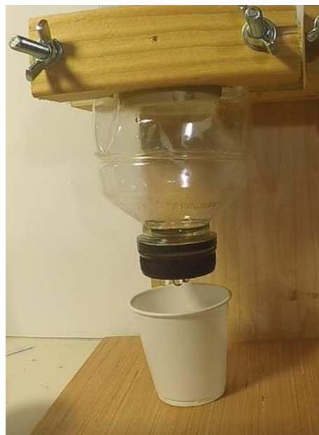
Figure 32. A bottle press to help with filtration using bottles and filter paper in the lids, which allows maintaining pressure on the bottles and use a laboratory filter or a coffee filter to extract the clays from the extract. This approach saves time because while pressing the bottles one can proceed with other tasks.
