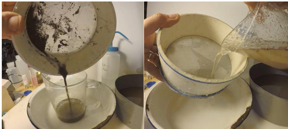
Figure 21. Left: Transferring the material from the 250 micrometer sieve (mineral mixed with POM) to a beaker for decanting of organic matter. Right: Decanting the 250 micron POM to a 250-micron sieve corner (at one edge of the sieve to facilitate moving the POM to a funnel for drying)
